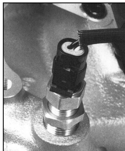
The Coolant Temperature sensor attaches to the harness with Connector J10.
