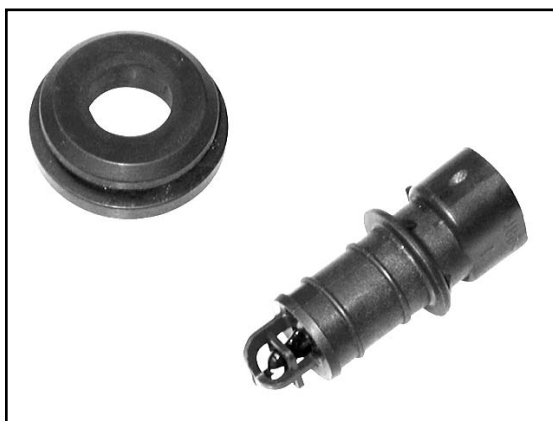
The Manifold Air Temperature sensor attaches to the harness with Connector J11.
